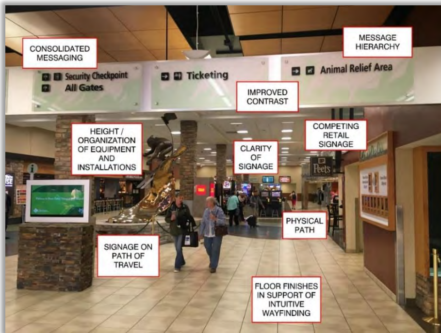
Figure 4-17: Main Lobby Wayfinding
